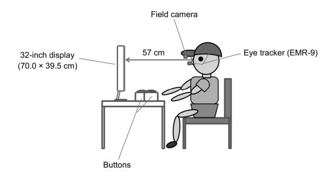
Note: The eye tracker system (EMR-9) with the 32-inch display was connected to the static image presentation system (Multi Trigger System) as shown.
